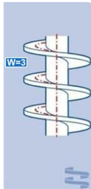
Number of windings W1, W2, Wn Picture -> W=3
