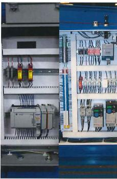
Microprocessors, variable frequency drives, and Category 3 Safety circuits are provided to fully integrate the control of the Man-On-Board Adjustoveyor.
