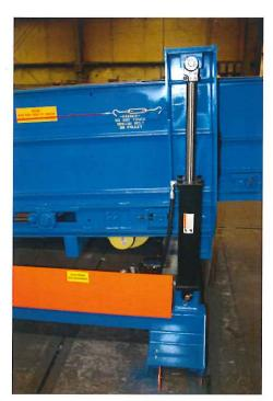
The elevation of the Adjustoveyor is controlled by two hydraulic lift cylinders and the Operator can move across the trailer and elevate to provide improved ergonomics and productivity.
