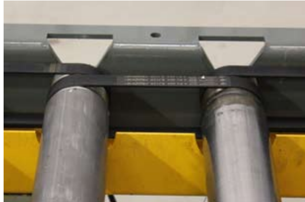
GUARD REMOVED TO ILLUSTRATE ROLL TO ROLL DRIVE BELT.
