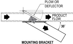
The 190-LRSS is equipped with mounting brackets to attach unit to side channel of 190-ACC, 190-ACZ, or 190-LR.
